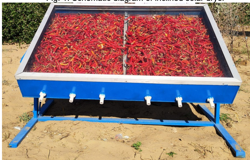
Fig. 2: Drying of red chilli in the inclined solar dryer
