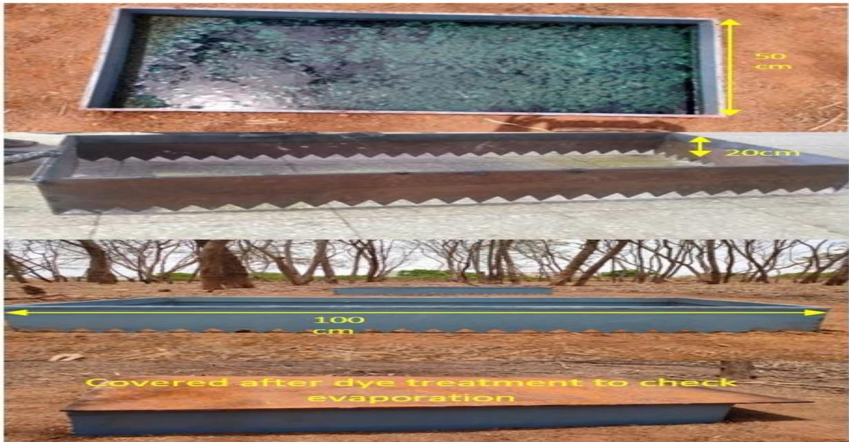
**Figure 1:** Iron frame fabricated for preferential flow study
