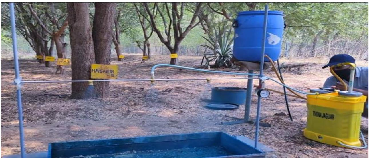
**Figure 2:** Application of Dye- water with power sprayer
